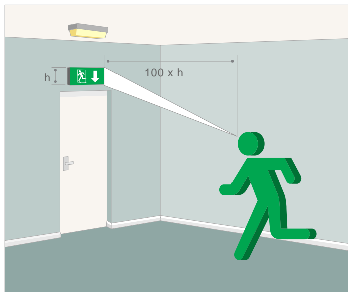
Externally illuminated signs - 100 x the panel height
