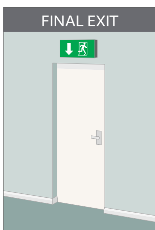
At each exit door
